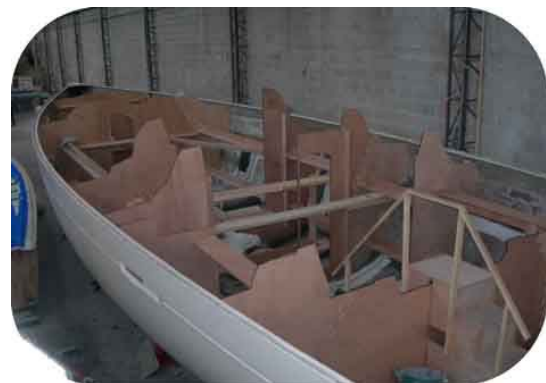
SECOND STEP : BULKHEAD AND FURNITURE IN THE HULL LAMINATED
