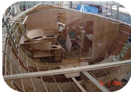
FIRST STEP : BULKHEAD AND FURNITURE BUILD IN THE SIMULACRE
